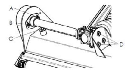
Adjust the drive belt tension. The correct belt tension is achieved when the belt can be deflected by the belt thickness about 10mm at the centre point between the pulleys.
